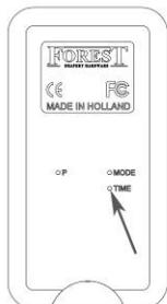
PRESS TIME FOR ~7SEC. UNTIL DIGITS STOP BLINKING → FINISHED
