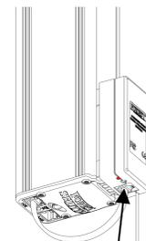
press and hold the program button for 10 seconds until led starts blinking
