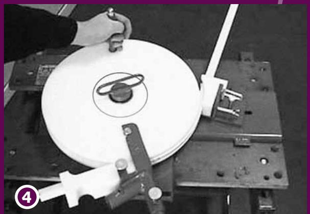
4 Tighten the screw on the Guide-Wedge. Start bending by turning the handle until the required angle is reached. For two curves in one track, measure from the outside of the track to the measurement line (F). This will create the distance from the outside of the track between the two curves.
