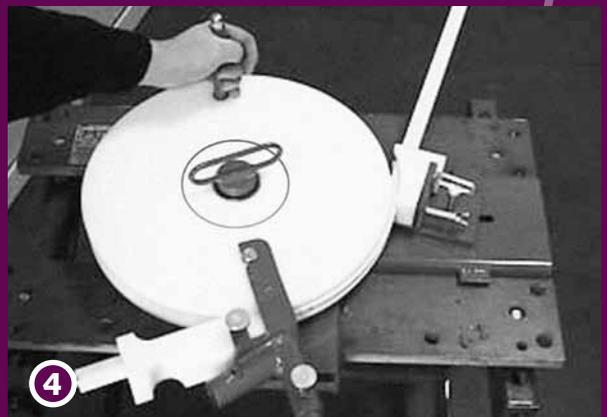
4 Tighten the screw on the Guide-Wedge. Start bending by turning the handle until the required angle is reached. For two curves in one track, measure from the outside of the track to the measurement line (F). This will create the distance from the outside of the track between the two curves.
