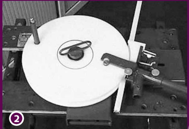
2 Insert the track from the backside of the Bending tool, between the Bending Dye (A) and the Bending House (E). Place the handle (D).
