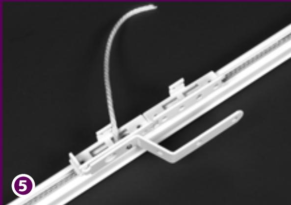
Determine the cord length by pulling the cord. Pull at the end to reduce the drop height, pull at the loop to increase the drop height. Screw the half cord connector tight to position the cord drop height (with CCS®: the second cord connector in the double construction).
