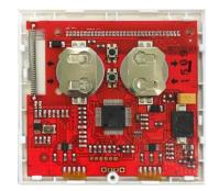
put in the two batteries mind the right polarity
